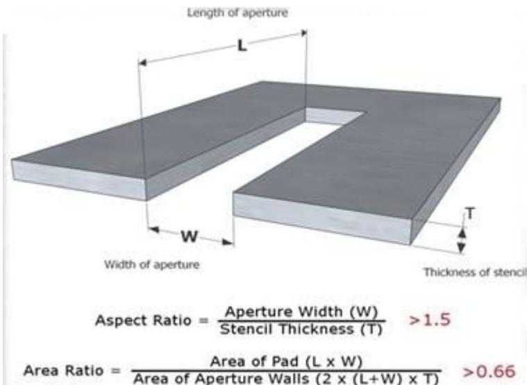
A 0.100 mm (4-mil) thick stainless steel stencil is recommended. When these stencil design requirements conflict with other required SMT components in a mixed technology PCB assembly, a step-down stencil process may be utilized in compliance with IPC-7525 [4] design standards.
