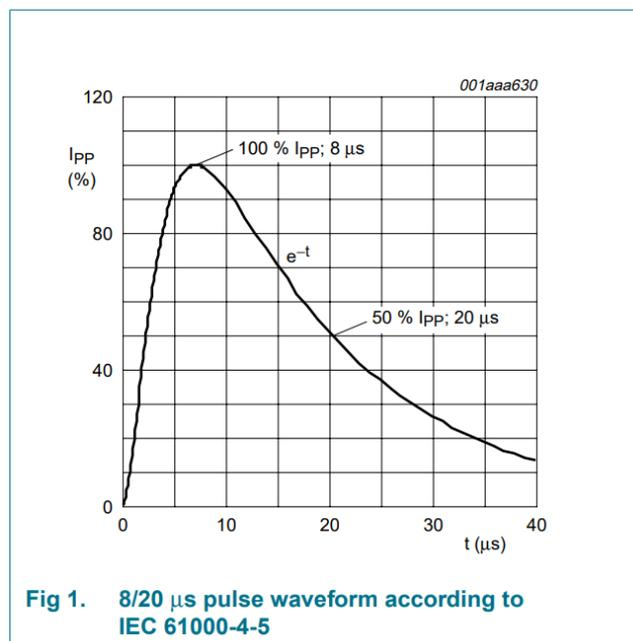
Fig.3 - Pulse Waveform
