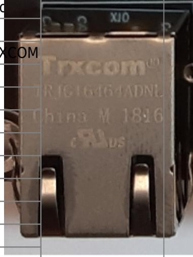
A photograph of the physical X10 Ethernet connector. The connector is a metal housing with two mounting holes at the top. The brand name "Trxcom" and part number "TRJG16464ADNL" are embossed on the side of the housing. The text "China M 1816" and "cTbus" are also visible. The connector is shown from a slightly angled perspective, highlighting its physical construction.
