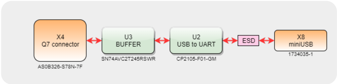
Q7Base USB debug console USB Connector (USB to UART console)
